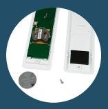
Replace the old battery with a new CR2430 battery. Then replace the back cover and tighten the screw by turning clockwise.
