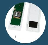
Gently pry open case to reveal the battery. Slide out the old battery.
