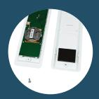
Gently pry open the case to reveal the old battery. Slide the old battery out.
