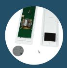
Insert a new CR2430 battery. Replace the back cover and tighten the screw by turning clockwise.
